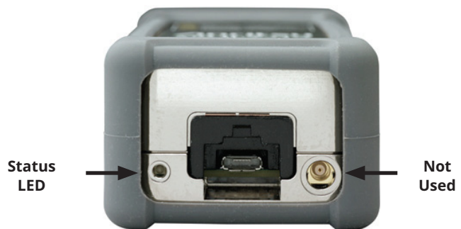
Micro USB Connector With Latch
